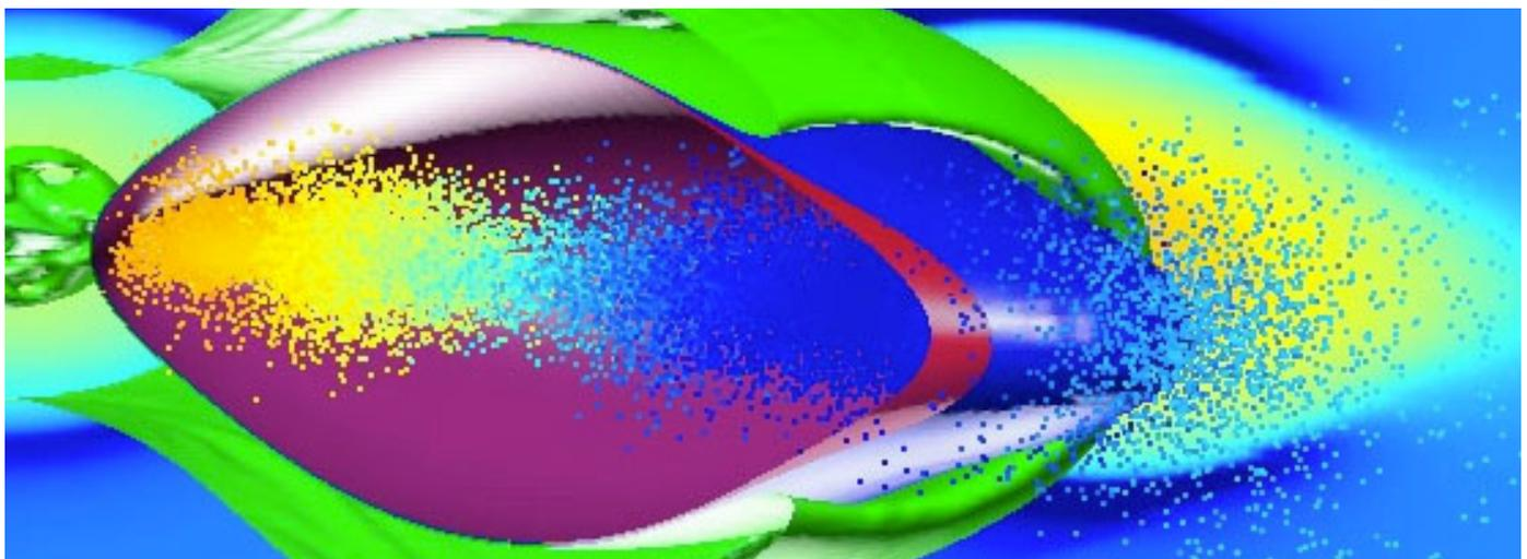
This simulation depicts two electron bunches – containing 5 billion to 6 billion electrons each – that were accelerated by laser generated plasma inside an oven of hot lithium gas during experiments at SLAC.
