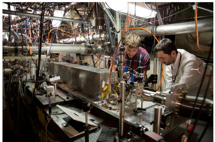
SLAC researchers monitor pairs of electron bunches sent into a plasma inside an oven of hot lithium gas at FACET.
