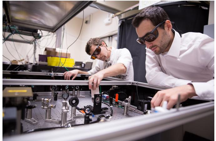
SLAC researchers use a laser table at FACET to create a plasma used for accelerating electrons to high energies in a very short distance.
