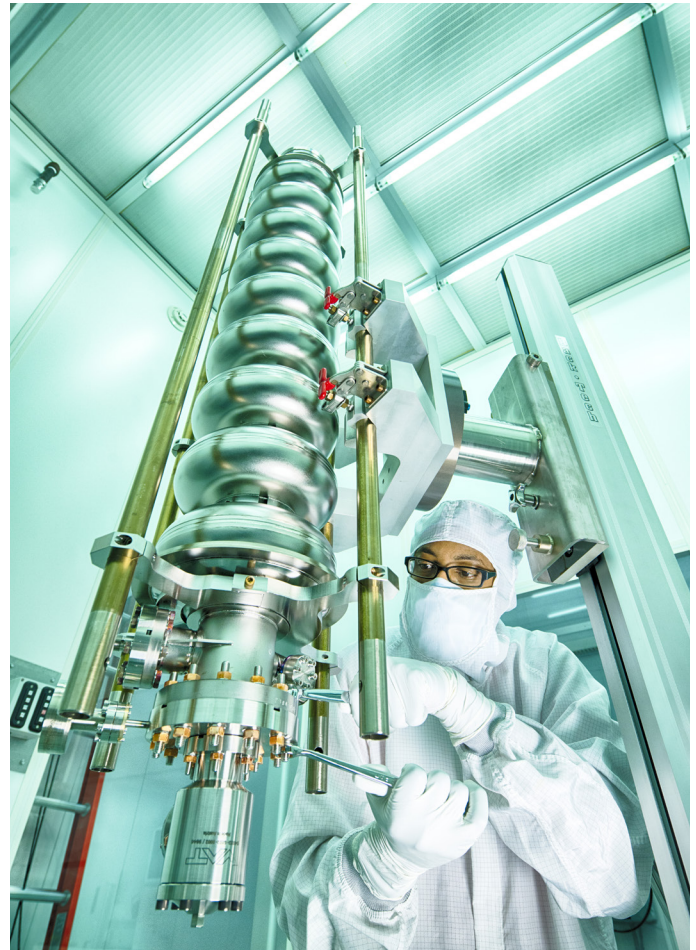
Cooled to minus 456 degrees Fahrenheit, these niobium cavities allow radiofrequency fields to boost electron energies without electrical resistance. Cryomodules—consisting of eight niobium cavities each—are a key component of LCLS-II's superconducting linear accelerator. (R. Hahn/Fermilab)
