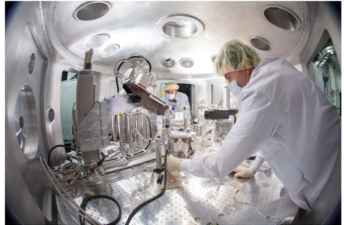
Scientists prepare for an experiment at SLAC's Matter in Extreme Conditions (MEC) station, part of the LCLS X-ray laser. They used this MEC station to create and measure the properties of ultrathin sheets of superheated aluminum as it transitioned into warm dense matter.
