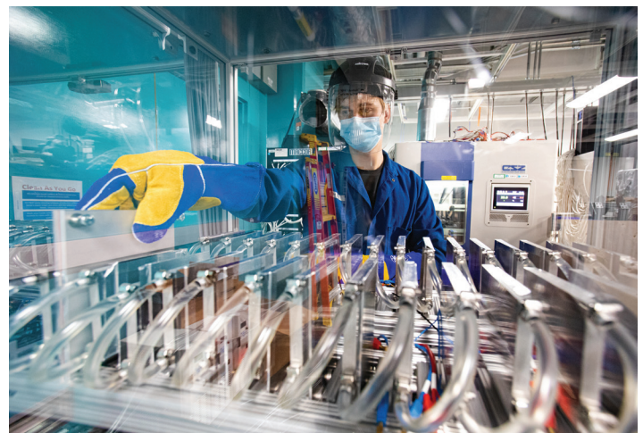
Staff engineer Bruis van Vlijmen sets up cell cooling plates in the Battery Informatics Lab at SLAC.
